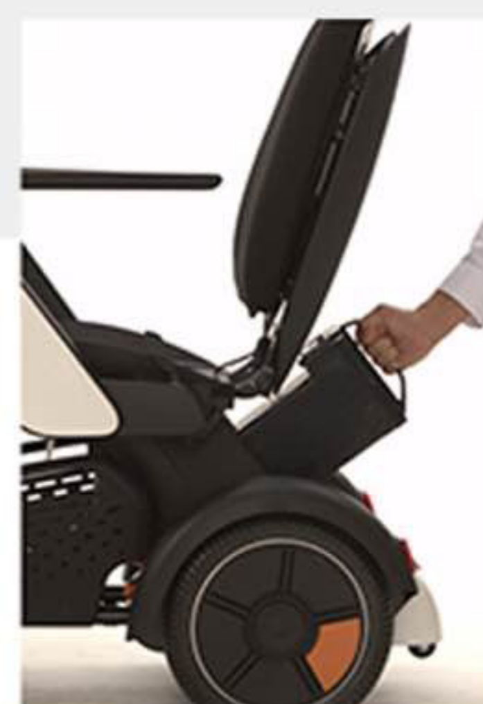
1/ Disconnect the power and pull out the battery
