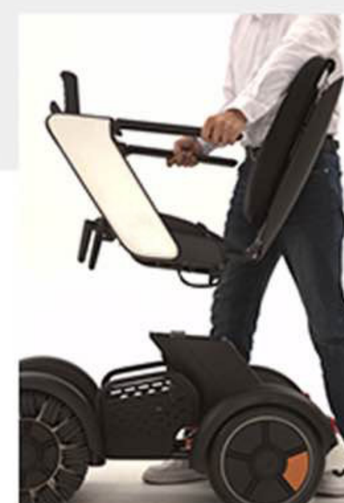
2/ Unlock the carabiner and remove the upper part of the seat
